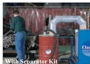
The 200 litre Separator Kit is ideal for removing large quantities of swarf and chips or for cleaning coolant from large sumps. It includes wheels, lever lock lid and the connecting duct.
