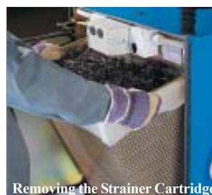
The Strainer Cartridge will hold up to 60 litres of swarf and chips and simply slides out. Various media screen inserts are available to suit different coolants, including a 300 micron mesh screen and a 25 micron polymer sheet.
