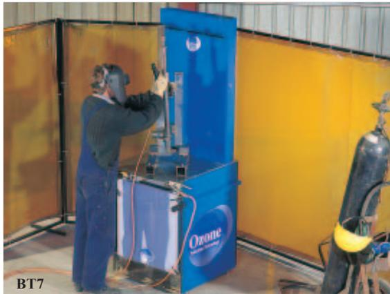
Model BQ7 has back-to-back workstations on the one Bench Cleaner. In this configuration the filtered air discharges to the side, away from both welders. An outlet silencer can be connected as shown, to further reduce the already low noise level.
