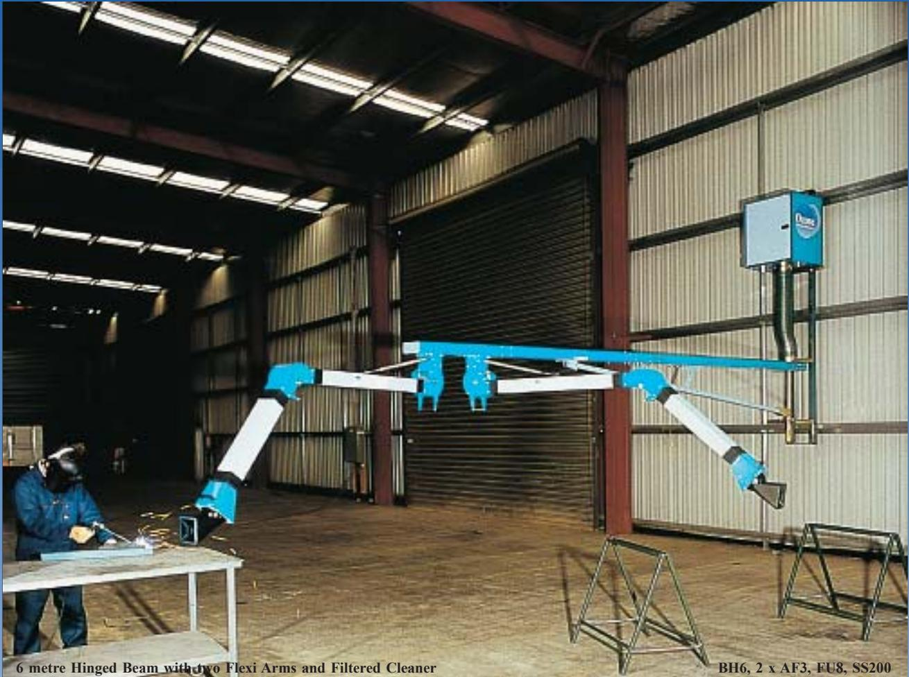
6 metre Hinged Beam with two Flexi Arms and Filtered Cleaner
