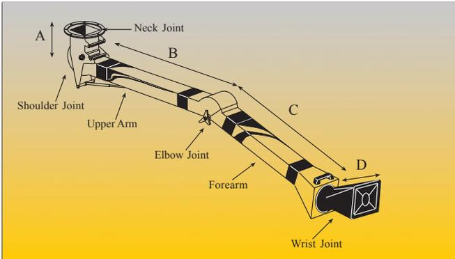
The low pressure drop design of the smoothly contoured Arm allows high airflows to be achieved by compact, power efficient extractors. In multi-arm systems, ducting design and extractor selection is now much simpler. Unlike conventional arms with flexible hose, the Ozone Flexi Arm does not “pinch” when folded up, so performance remains high no matter what position the arm is in.
