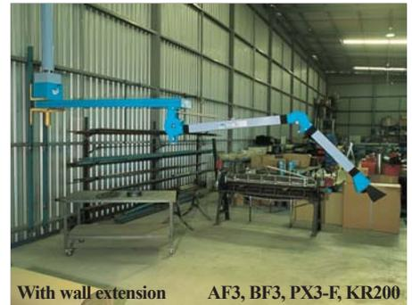
Mounting two Flexi Arms on a Duct Kit, which in turn is directly connected to an Extractor, is an ideal system for side-by-side work stations.
